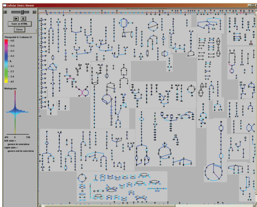
Fig. 6.1 The Cellular Omics Viewer. This image shows an E. coli gene expression dataset painted onto the E. coli metabolic network. The color assigned to each line (reaction) corresponds to the expression level of the gene coding for the enzyme that catalyzes that reaction. The controls in the upper left allow the user to stop and start animated displays within this diagram
