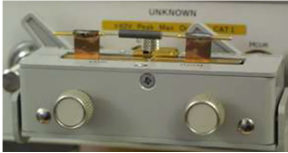
Fig. 15 Piezoelectric sample placed between electrodes in the HP sample jig
