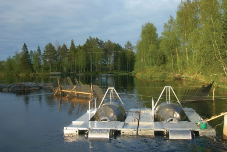
Fig. 20.3 River Sävarån smolt traps with their lead-arms that guide downstream migrating fish toward(s) the traps, as seen from downstream
