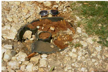
Fig. 6 Examples of the French 1947 AT landmine in Southern Lebanon. (Photo: Bactec.)
