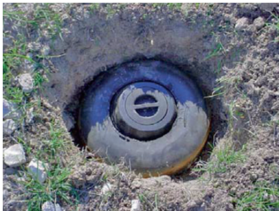
Fig. 6 Examples of the French 1947 AT landmine in Southern Lebanon. (Photo: Bactec.)
