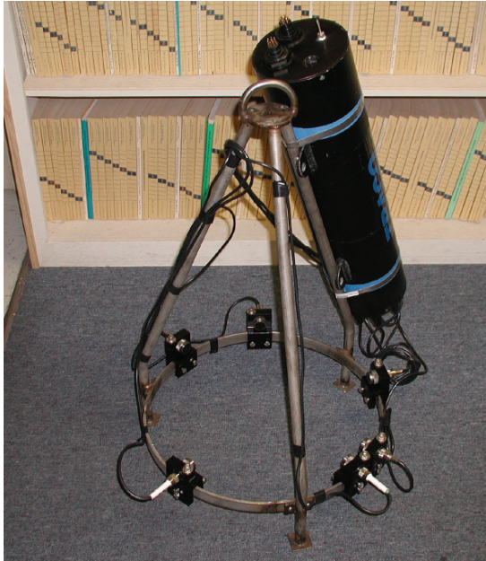
Fig. 17.3 A circular frame holds several broadband transducers aimed at the center of the circular plane area. The long black cylinder is a pressure case for electronics. This configuration uses two transmitting transducers in order to cover a wide frequency band ( bottom right ). Pulses are directed across the diameter of the measurement plane. Multiple receiving transducers are located at known, adjustable, angles in the horizontal plane and are used to intercept echoes when one (or more) scatterer is detected in a very small volume in the center of the circle formed by the frame
