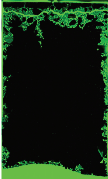
Fig. 11.4 Impregnated core, showing delamination at 7 to 12 mm from the top surface. The wavy lower core face is due to pouring on plastic foil on sand bed. Core dimension: 100 × 170 mm
