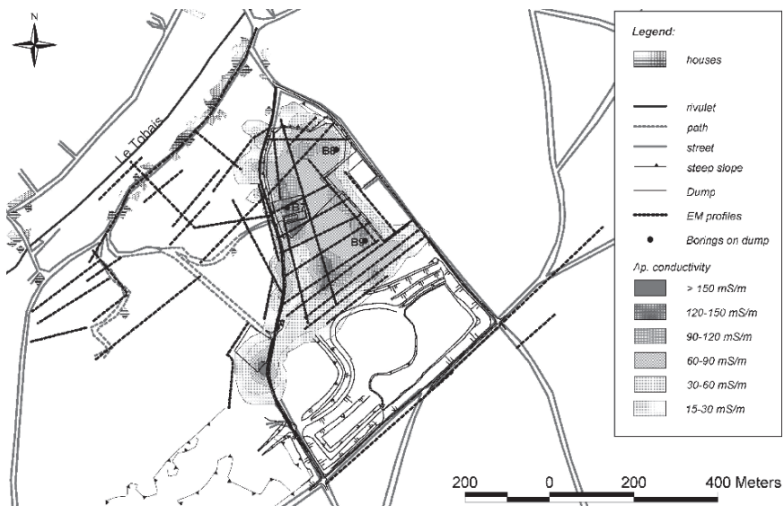
Fig. 12.9 Ground conductivity at a subsurface industrial dump site, mapped based on electromagnetic prospection with S = 20\text{ m} (Adapted from Walraevens et al. 2005)
