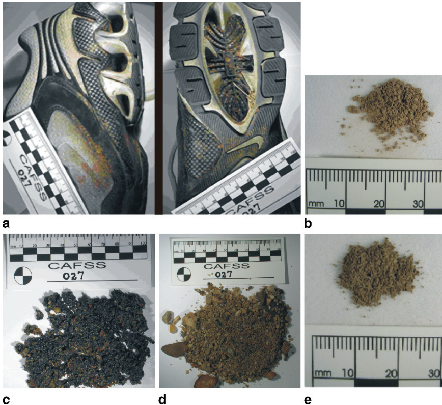
Chap. 8 Fig. 2 Soil samples associated with the hit-and-run case study. (a) Shoes from suspect; (b) sample scraped from the shoe; (c) control soil specimen from the river channel; (d) control soil specimen from the bank of river and (e) the <50µm fraction separated from this sample
