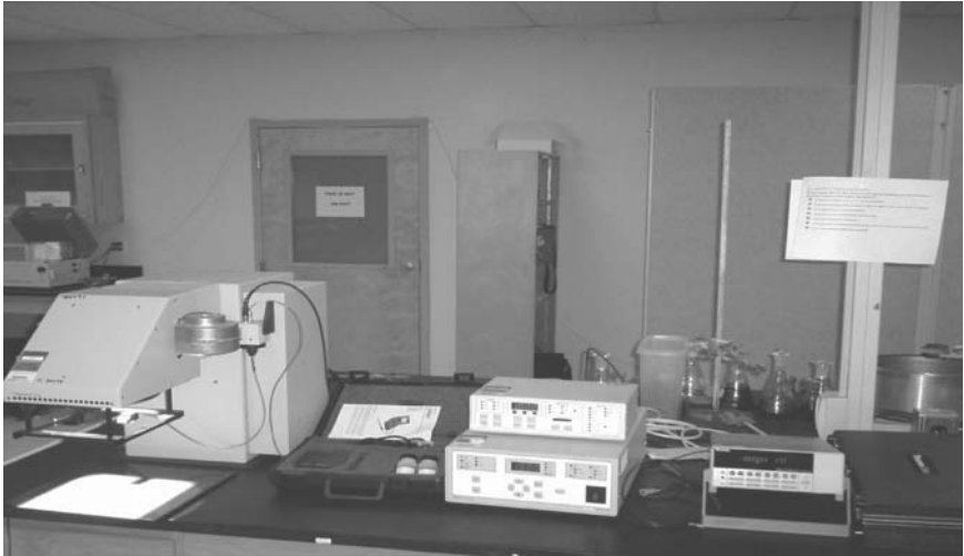
Fig. 7 Solar simulator and its controls along with the electrometer at Research Center for Cutting Edge Technologies (RECCET)
