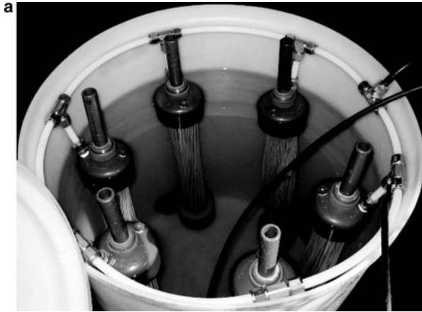
Fig. 2a Six Zenon ZeeWeed 10 UF pre-treatment membranes connected in parallel
