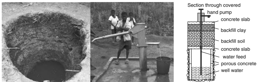
Fig. 1 Open (unprotected) and covered (protected) shallow wells in Malawi
