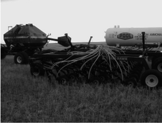
Fig. 31.6 The Day's sowing canola into wheat stubble with their SeedHawk toolbar and Morris air tank
