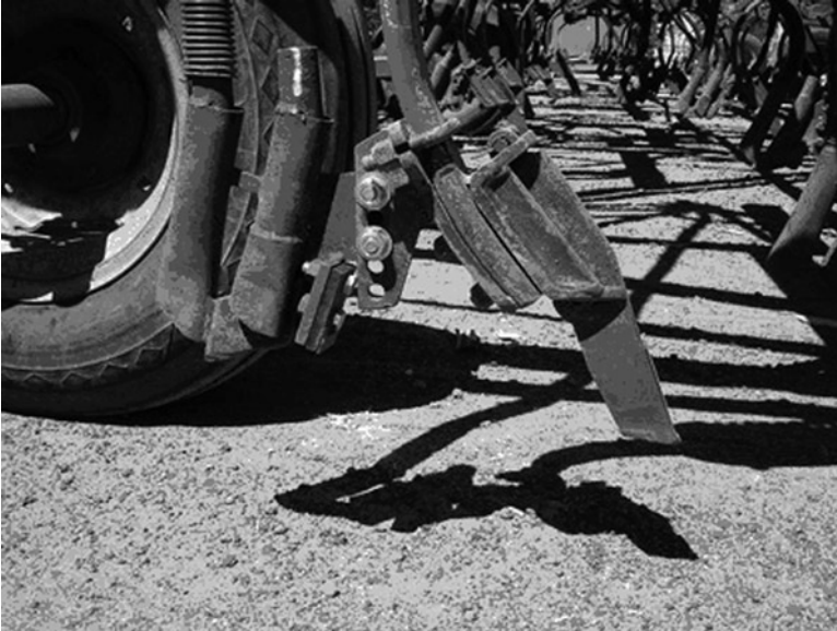
Fig. 39.4 Tine sowing systems are limited by the amount of crop residue they can handle
