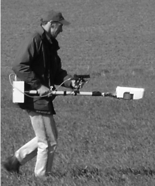
Fig. 34.7 The N-Tech GreenSeeker® RT 100 being used to measure an N-Rich strip in Tarlee, South Australia
