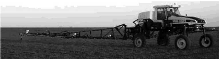
Fig. 34.6 The N-Tech, RT 200 with 6 Greenseeker® sensors mounted across a self propelled boomspray in Virginia, USA
