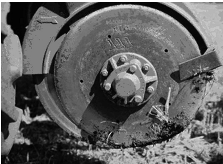
Fig. 39.6 Brazilian disc seeder designs can seed into high residue conditions (7 t/ha of plant residues)
