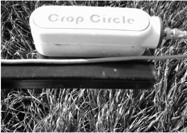
Fig. 34.8 The Crop Circle ACS-210 being used to measure the NDVI in barley in South Australia
