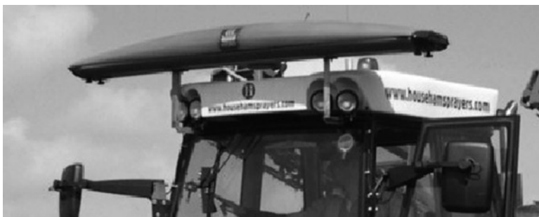
Fig. 34.5 The Yara N Sensor mounted on a Househam self-propelled boomspray
