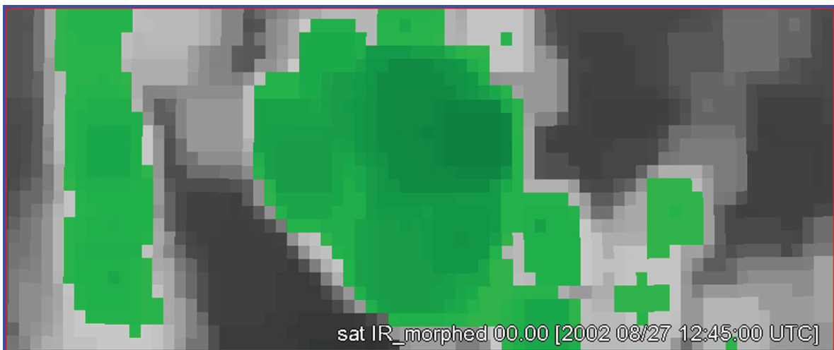
Fig. 16.8 Spatial dilation and erosion operations may be performed by replacing a pixel with the maximum or minimum of the values of its neighbors
