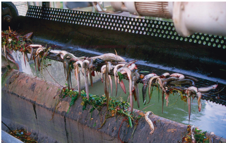
Fig. 4.5 Eel collected from the trash rack at the Wahnhausen power station at the river Fulda in Hessen, Germany (photo by Adam B)
