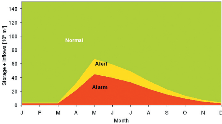
Fig. 14.14 Triggering levels for normal, alert and alarm conditions
