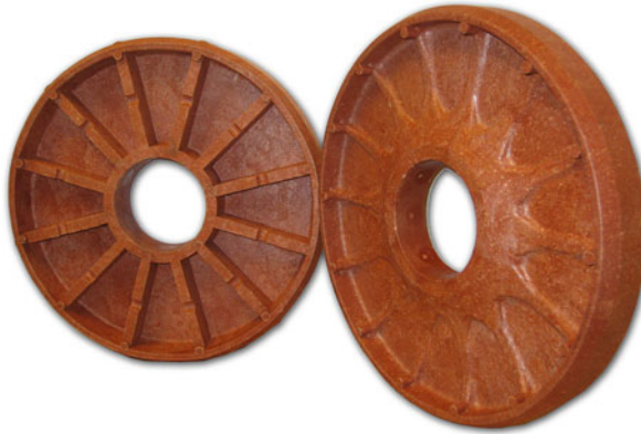
Fig. 37.6 Left – First version of the core plug. Right – Final version of the core plug
