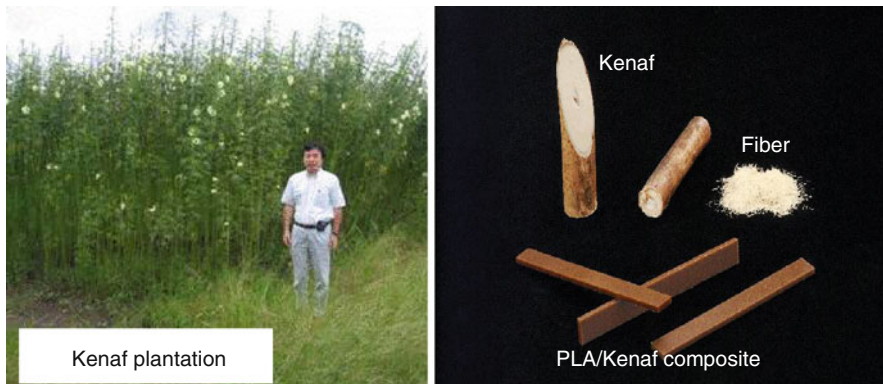
Fig. 62.2 Kenaf, kenaf fiber, and molded PLA/kenaf composite
