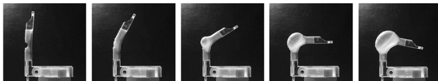
Fig. 3 Monotonic deformation behaviour of a pneumatically driven compliant mechanism made of silicone rubber
