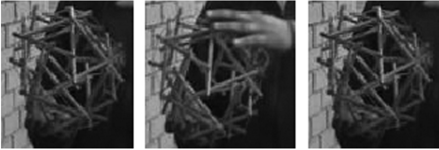
Fig. 1 Tensegrity system built with cables, subjected to a perturbation
