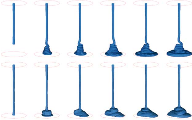
Fig. 8. Jet buckling in a cavity. Shape of the jet at time t = 0.125 s (col. 1), t = 0.45 s (col. 2), t = 0.6 s (col. 3), t = 0.9 s (col. 4), t = 1.15 s (col. 5), t = 1.6 s (col. 6), Newtonian fluid (row 1), viscoelastic fluid (row 2).
