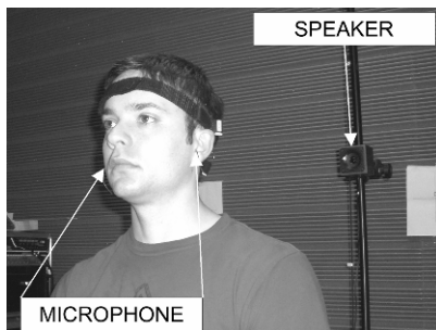
Fig. 3: Empirical HRTF measurement at FIU.
