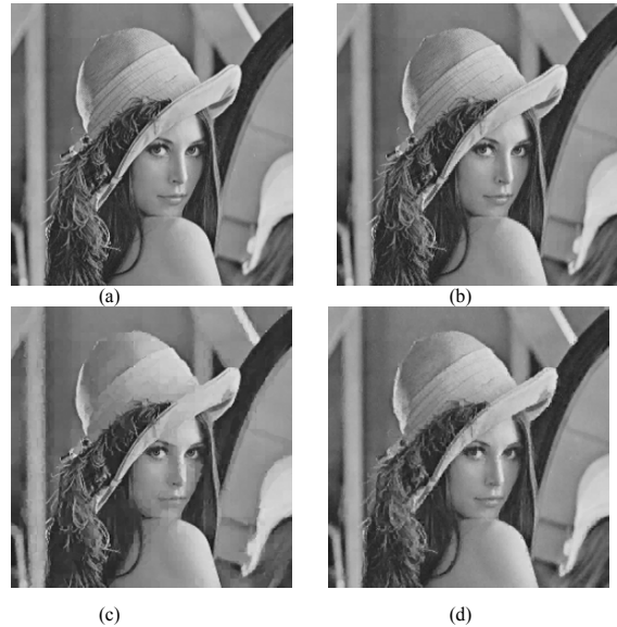
Figure 3 – Results of the probabilistic search method. (a) – Fractal compression, exhaustive search, low threshold, small range blocks, maximal compression time (b) – Probabilistic search, same threshold and range blocks, 75% time reduction, small reduction in image quality (c) Time reduction by using the traditional method with larger threshold, massive quality reduction (pixelization) (d) Time reduction by using the traditional method with larger range blocks, massive loss of details (e.g. the distortion of the eyes)
