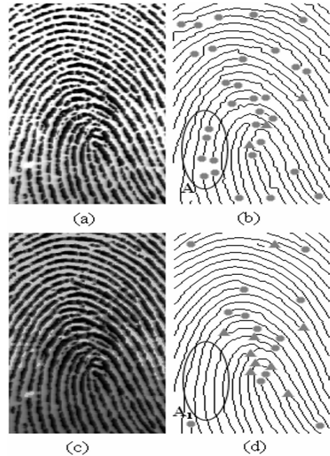
Fig. 4. Demonstration of proposed technique: bullets are endpoints and triangles are bifurcations: (a) Original image (c) enhancement algorithm result (b) thinned original image with 52 extracted minutiae (d) thinned enhanced image with 30 extracted minutiae
