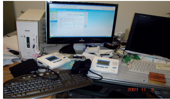
Fig. 4. Test Equipments (WebDoc MX431, PC, PDA, PLC Modems)
