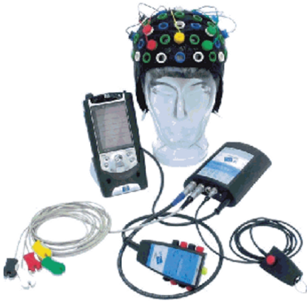
Figure 2.16. A g.tec head cap system for EEG recordings (Reprinted with permission from g.tec).
