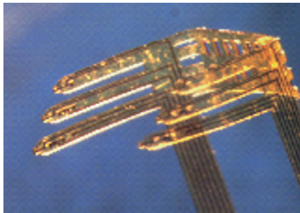
Figure 2.12. Photograph of a polyimide-based microelectrode array for intracortical implantation. The semitransparent polyimide substrate can be folded to achieve multishank arrays. The metal connecting lines are visible (Photograph provided by Daryl Kipke of the University of Michigan Center for Neural Communication Technology; reprinted by permission from Encyclopedia of Sensors [Burmeister and Gerhardt, 2006]).
