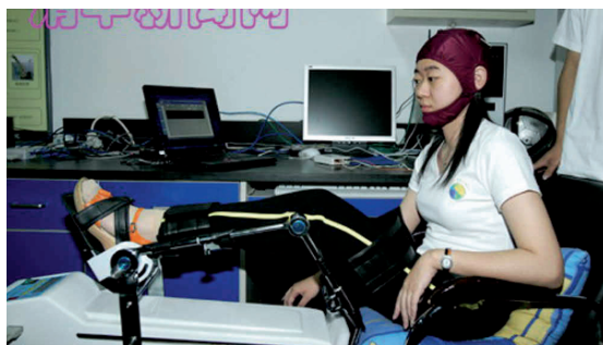
Figure C.29. The sensors in the EEG cap are used in EEG-feedback rehabilitation equipment.
