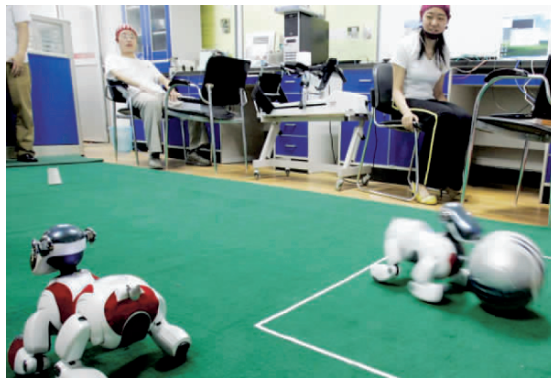
Figure C.23. Motor imagery-based BCI for robotic dog control.
