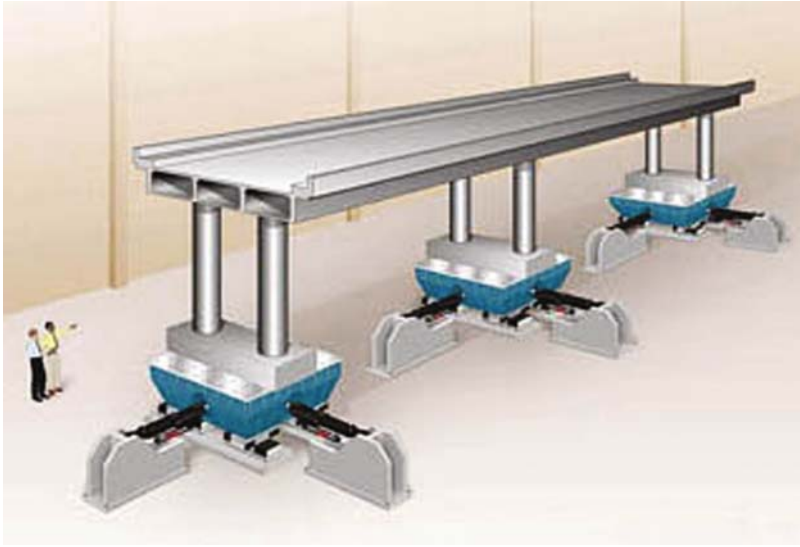
Fig. 7 NEES Three 2DOF Shaking Tables at the University of Nevada (Reno)
