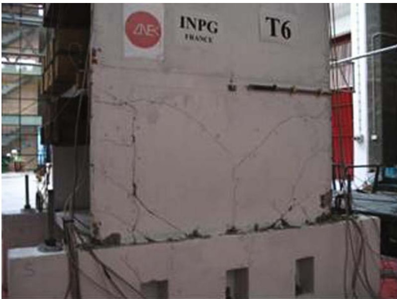
Fig. 17 Experimental damage pattern for T6 motion
