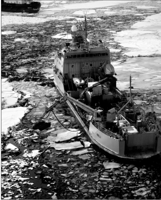
Figure 5. Brush drum on arm.
