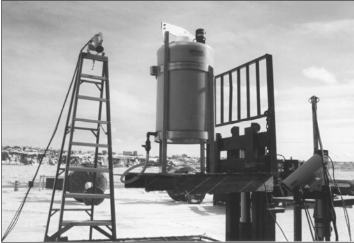
Figure 2. Tank used for sediment/water mixture and introduction onto the oil slick.
