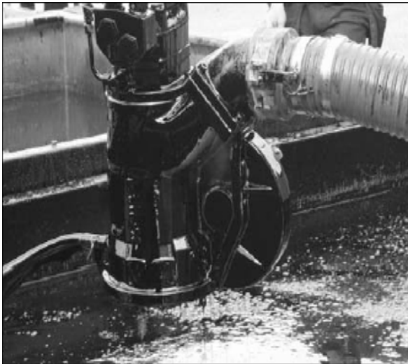
Figure 4. Screw auger pump.
