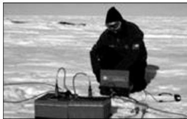
Figure 6. Ground Penetrating Radar (GPR) system in the Arctic. Source unknown.
