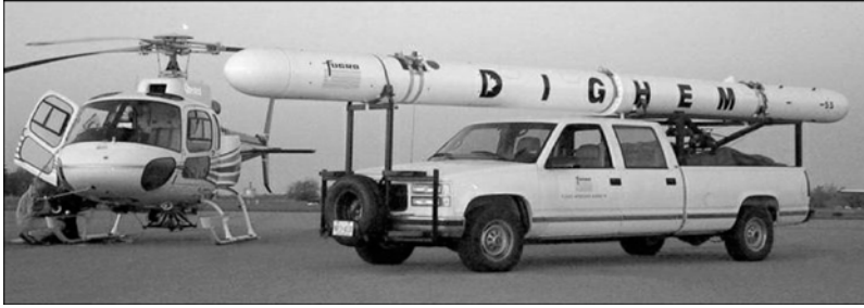
Figure 5. Electromagnetic induction sensor. Photo by Fugro Airborne Surveys. Source unknown.
