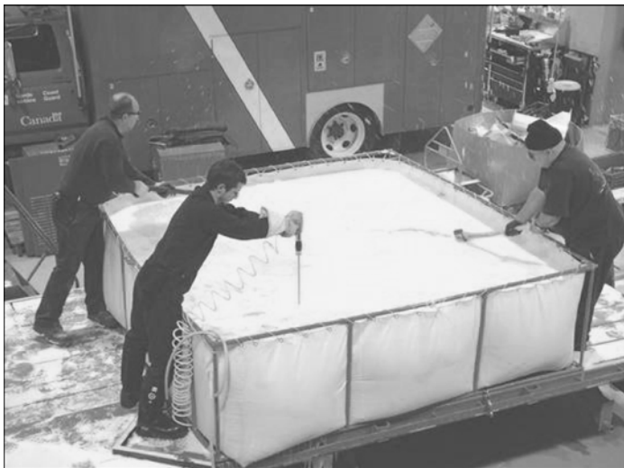
Figure 1. Top view of the basin filled with frozen brackish water. The ice cover is broken down before the experimentation.
