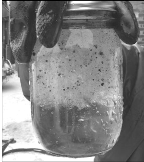
Figure 8. oil droplets trapped inside the slush ice matrix after sampling.
