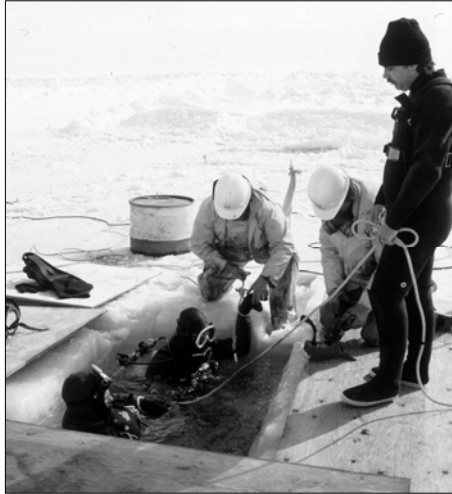
Figure 2. Measuring oil under ice roughness in the Canadian Arctic.
