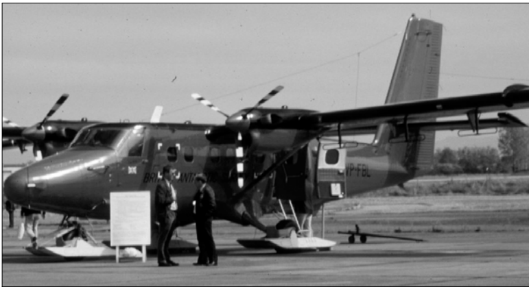
Figure 7. British Antarctic survey Twin Otter with radio echo sounding system Strasbourg, France.
