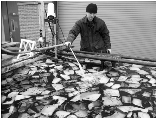
Figure 3. The entire oil slick is treated with a sediment/water mixture introduced uniformly onto the surface of the slick.
