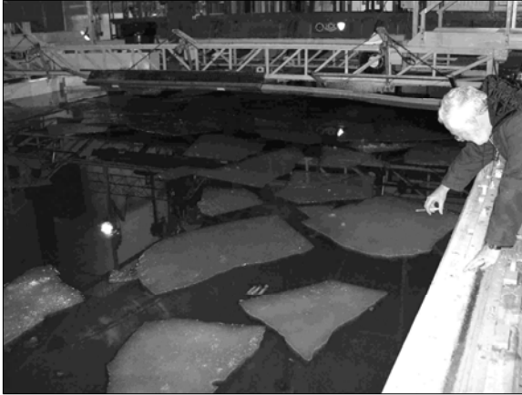
Figure 7. Applying herder around periphery of slick.
