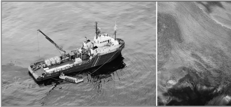
Figures 4 and 5. (4) Recovery of the remaining emulsion from slick A with the sweeping arm in very calm seas two days after release. (5) Aspect of the emulsion.
