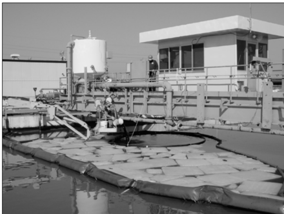
Figure 15. Adding crude oil to containment ring.
