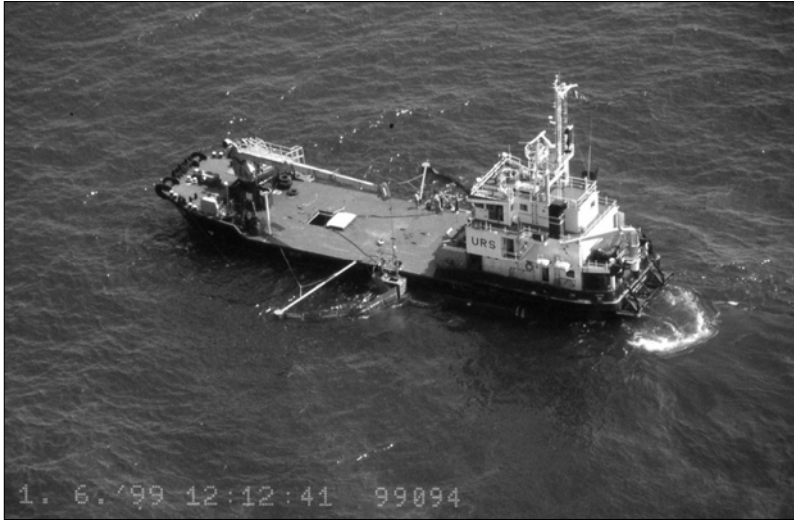
Figure 3. Multipurpose vessel equipped with oil-recovery systems under contract of the Belgian authorities (1994–2001).
