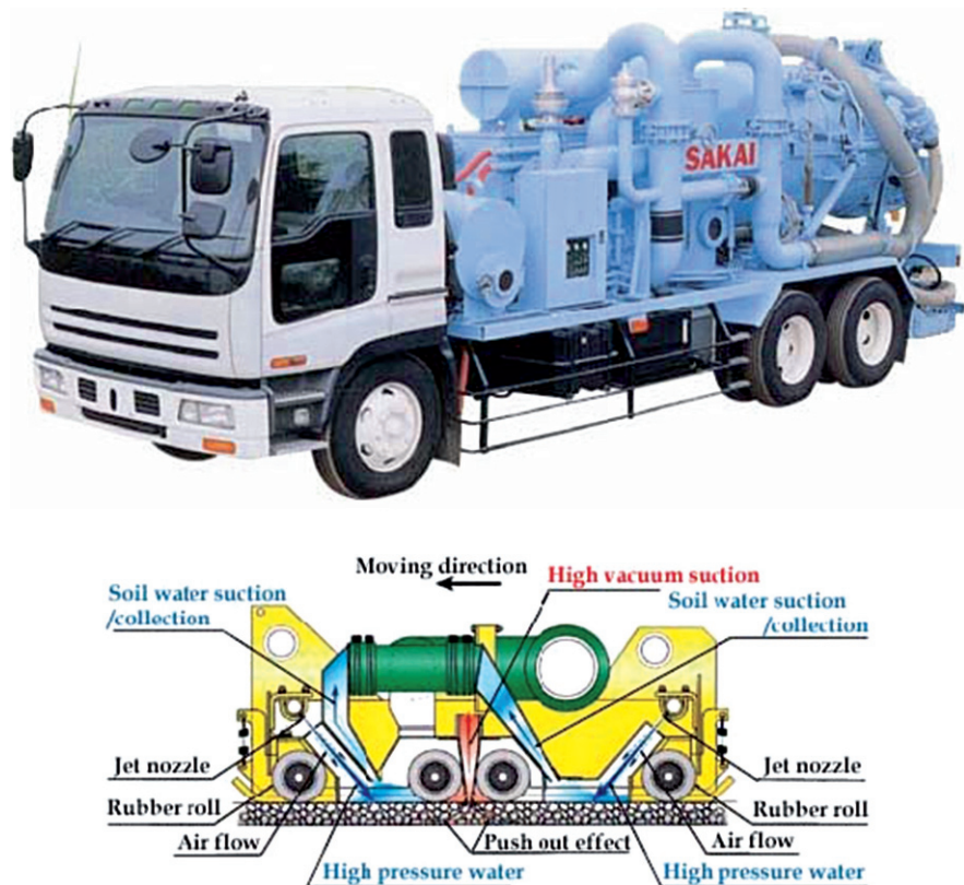
Fig. 5.18 Porous asphalt cleaning machine and diagram of active part. Reproduced by permission of Sakai Heavy Industries
