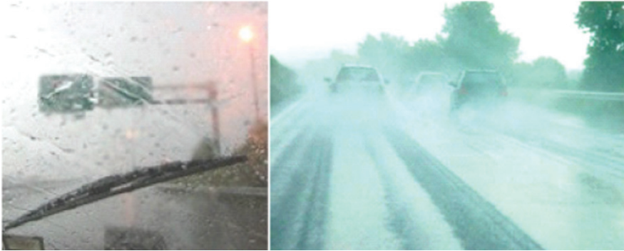
Fig. 5.15 (a) bad road visibility conditions (b) hydroplaning and ‘splash and spray’ (Erkens, 2005). Reproduced by permission of N. Kringos
