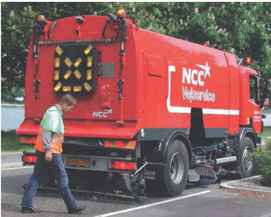
Fig. 5.17 Porous asphalt cleaning machine. Reproduced by permission of the Danish Road Institute
