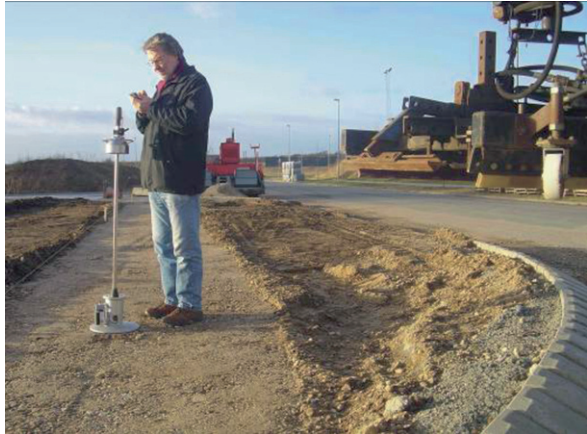
Fig. 10.7 Portable FWD. Photo courtesy of Grontmij/Carl Bro A/S. Reproduced by permission of Carl Bro Pavement Consultants A/S
