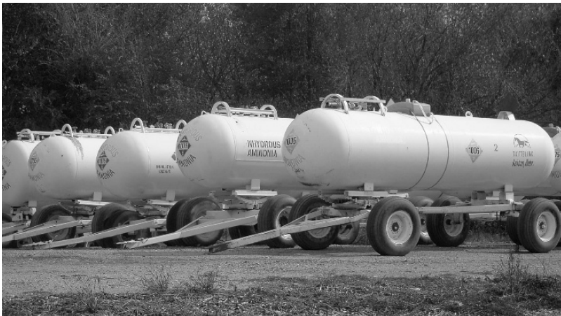
Fig. 13.2 Anhydrous ammonia tanks in a rural part of the state. Photo: Kevin Romig
