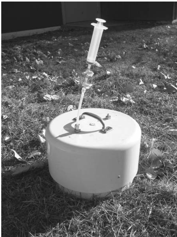
Fig. 12.1 Gas sampling chamber positioned on collar with syringe equipped with stopcocks attached to 1/4" bevel-a-line tubing sample port. A 1/4" diameter Swagelok fitting (on the right) serves as a vent
