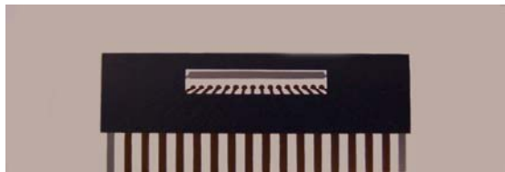
Figure 4. Multiprobe chip with 16 gold working electrodes and gold stems.
