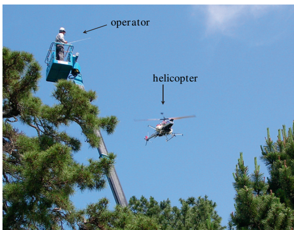
Fig. 4 Spraying with insecticide by remote-controlled small-scale helicopter
