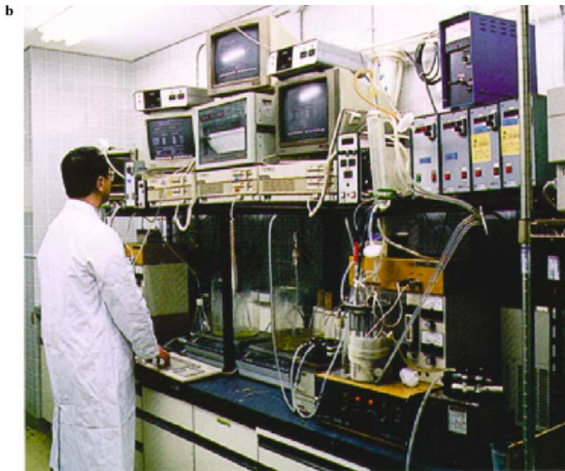
Fig. 1.1 (a) Dr. Hiroshi Kuriyama working with a continuous culture of Saccharomyces cerevisiae : (b) The continuous culture system. The impellers were driven by a 24 V motor (K; green line) and controlled by a power supply(A). Temperature was measured using a Pt 100 probe (yellow line) and controlled (B) to a user set-point by a 333 W heater (pink line). A water jacket (at 10°C) consisting of rubber tubing wrapped around the glass vessel (G) provides cooling (not shown). pH was measured using a steam sterilizable gel electrode connected (cyan line) to a (continued)
