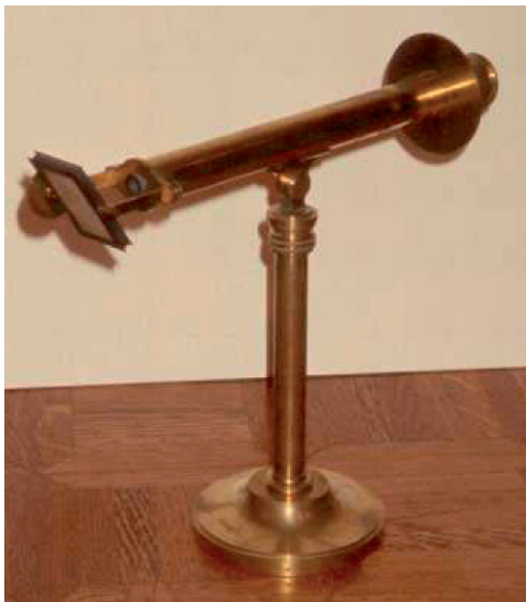
Fig. 7.1 The polarimeter which Arago used to demonstrate the laws of light polarized by reflection and refraction, now preserved at the Millington-Barnard Collection, the University of Mississippi, USA
