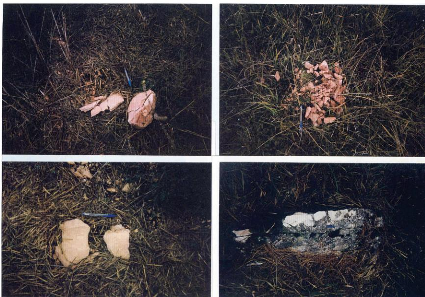
**Fig. 5** Typical pictures of isolated stones (fragile marly limestone) found throughout a 1-km<sup>2</sup> zone following the  $M = 6.0$  Colfiorito earthquake. The two original stones on the left were broken into several pieces while the one on the *upper right* was completely shattered. The rock on the *lower right* had its top partly scaled (the white areas), likely at impact. (After Bouchon et al. 2000.)
