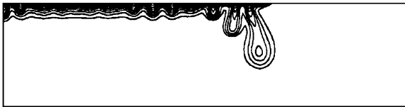
Fig. 10 Depicting the complex plume generated near the leading edge of a suddenly salted semi-infinite surface with suction (Wooding et al. 1997)
