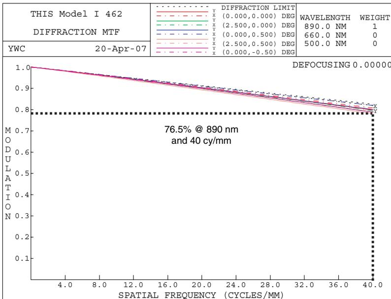
Fig. 6 MTF estimation for 890 nm
