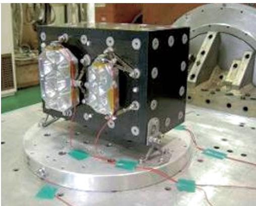
**Fig. 13** Random vibration test of SM
