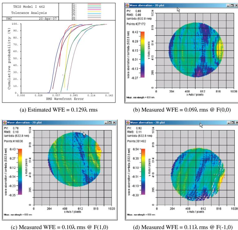
Fig. 11 Estimated and Measured WFE for M2 Alignment (a) Estimated WFE =  $0.129\lambda$  rms, (b) Measured WFE =  $0.09\lambda$  rms @ F(0,0), (c) Measured WFE =  $0.10\lambda$  rms @ F(1,0), (d) Measured WFE =  $0.11\lambda$  rms @ F(-1,0)
