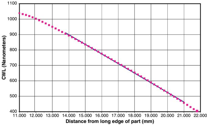
Fig. 3 Spectral range, dispersion and linearity of LVF
