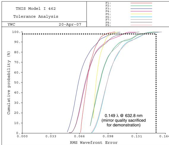
Fig. 7 WFE prediction for secondary mirror alignment
