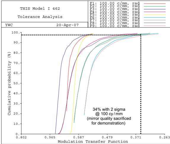
Fig. 8 MTF prediction for PAN in across-track direction
