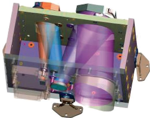
The box-type structure of the TIS system is based on honeycomb panels with composite face-sheets designed to minimize mass and to have enough stiffness. The reference planes for the optical surfaces are implemented with invar inserts through the honeycomb panels.
