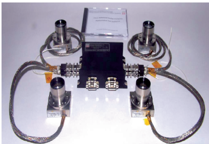
Fig. 4 The STR \mu ASC for the Swarm mission. Central: redundant electronics box. Each side can operate up to four camera heads
