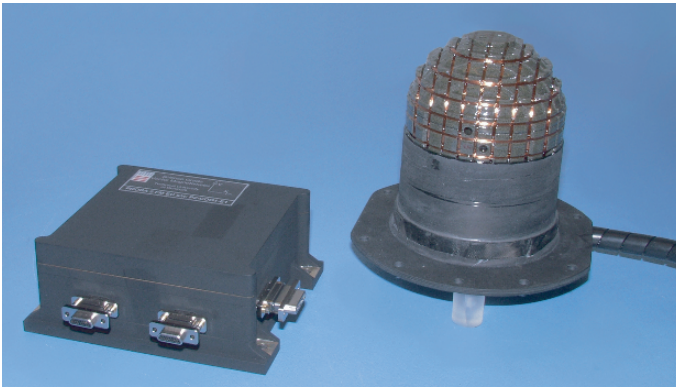
Fig. 3 The VFM magnetometer configuration for the Swarm mission. Left : redundant electronics box with Right : CSC sensor (shown with a CHAMP holder)
