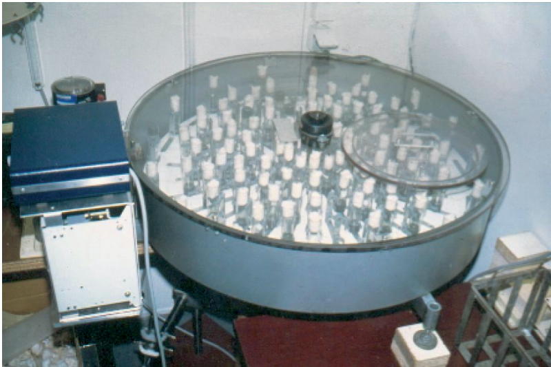
Fig. 1 Picture of the most commonly used centrifuge (1 m diameter). Flies are kept in their usual vials stored in the centrifuge. With a 102 rpm speed, the outer gravity level reaches 5 g
