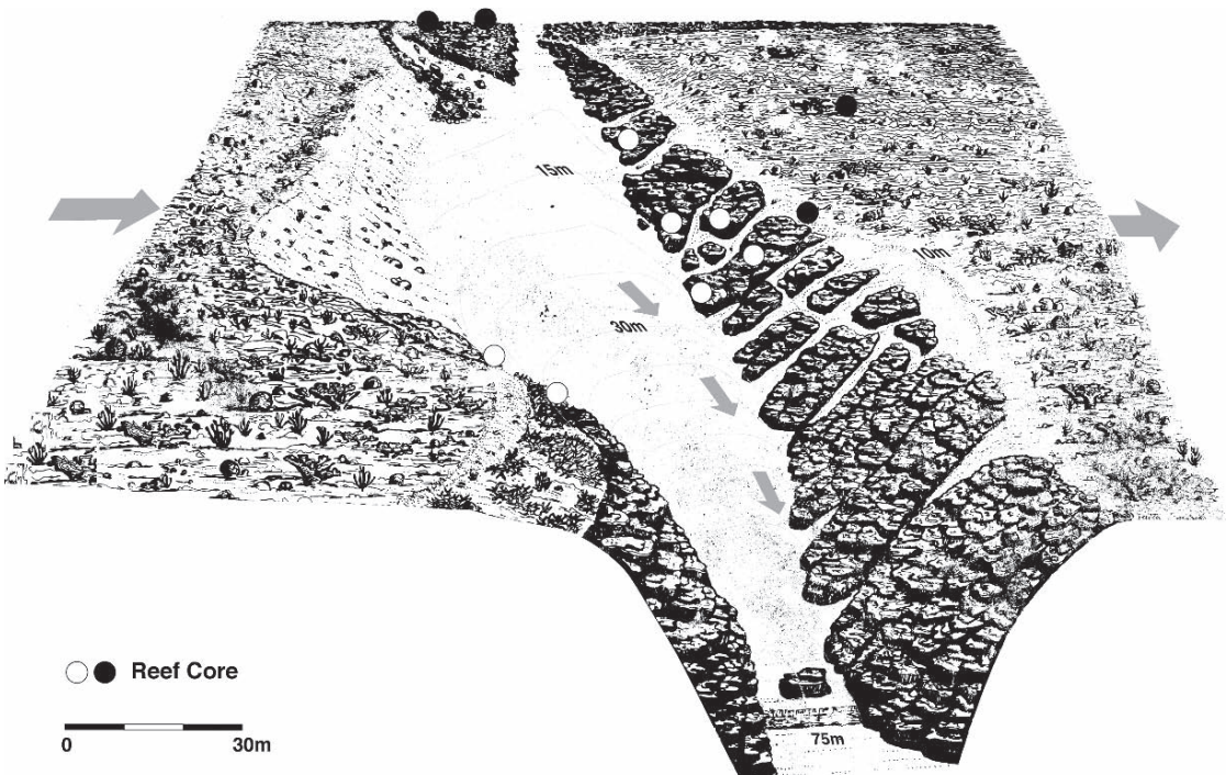
FIG. 7.28. Stylized block diagram looking up-canyon (south) at Salt River. This diagram is based on bathymetry and over 300 dives by the first author and colleagues. Sediment-transport pathways (gray arrows) and cores (black and white circles) are also shown. Figure 7.29 is based on the three seawardmost cores along the west (right) wall (After Hubbard 1989b by permission of West Indies Laboratory)
