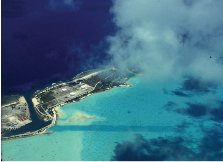
FIG. 17.22. The small boat harbor was originally open to the lagoon but was sealed by construction of a seawall. The small boat channel that was once used is evident but was closed off when the causeway connecting Wake Island (left) to Wilkes Island (right, with the three fuel storage tanks) was constructed. The overall best diving was in the immediate area on the outside reefs by this harbor. The wreck of an oil tanker is in shallow water by the harbor entrance and is colonized by corals
