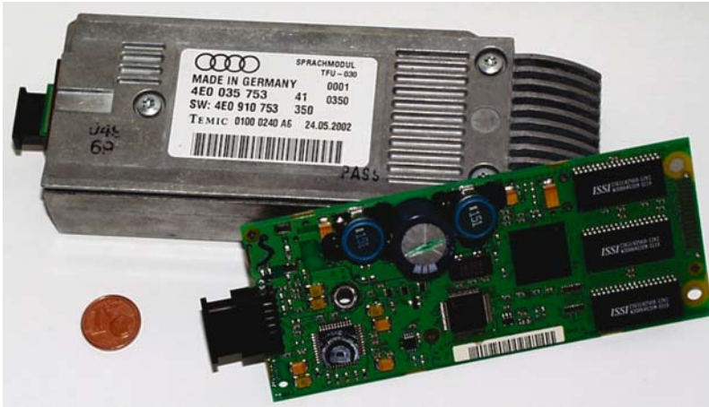
Figure 1. Hardware speech dialogue module.
