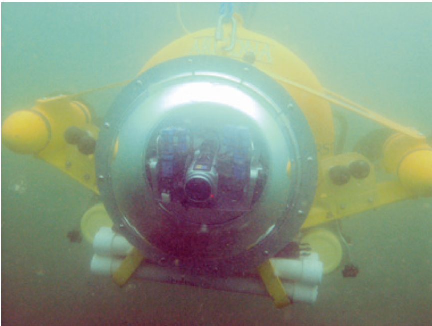
Fig. 20.7 Shadow during field testing in Prince William Sound. Shadow is a prototype submersible vehicle designed to remotely videotape a sonic-tagged benthic marine animal.
