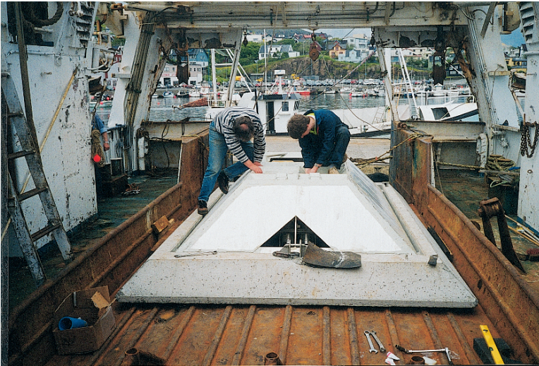
Fig. 1.7 Trawl-proof frame containing ADCP, double acoustic releases, ARGOS beacon, and buoyancy, on top of concrete anchor, is being made ready for deployment onboard R/V Magnus Heinason
