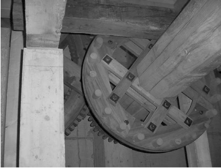
Figure 4: Gear Transmission of Le Tsáblo. Left: Gear on the First Shaft, which carries the Waterwheel. Right: Second Horizontal Shaft with One of the Two Wheels with Lateral Teeth.
