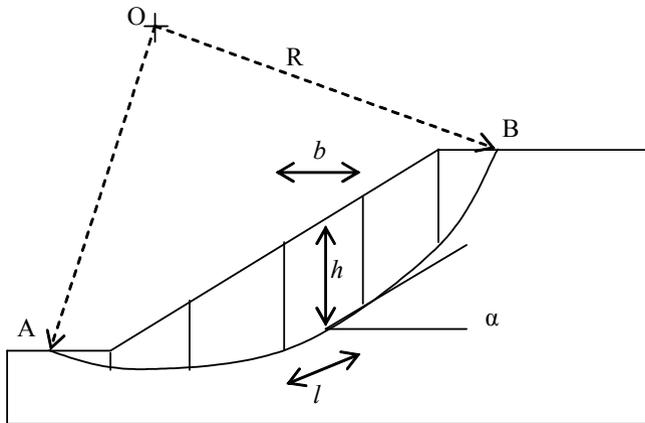
Figure 5-2. Method of slices. A circular slip surface of radius  $R$ , has centre  $O$  and intersection points at the ground surface of  $A$  and  $B$ . The soil mass above the slip surface is divided into a number of vertical slices of width  $b$  and varying height  $h$ . The base of each slice is assumed to be a straight line inclined at an angle  $\alpha$  to the horizontal and with a length  $l$ .
