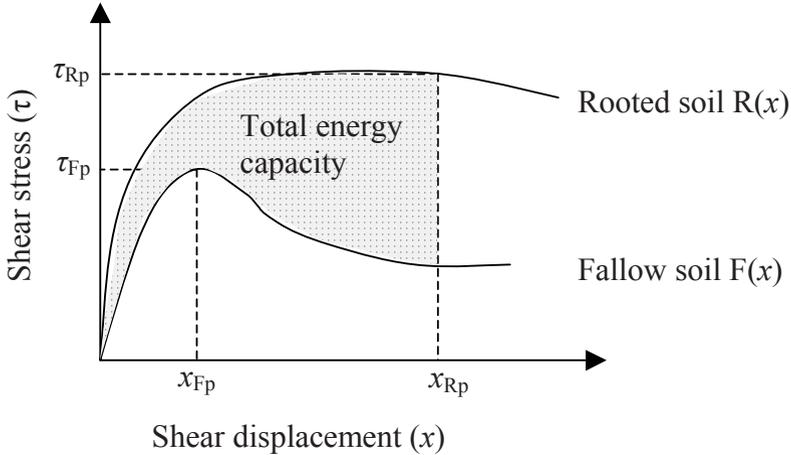
Figure 5-9. Ideal shear stress–displacement curves for fallow soil  $F(x)$  and soil with roots  $R(x)$ .  $x_{Fp}$  is shear displacement at the peak stress ( $\tau_{Fp}$ ) for fallow soil and  $x_{Rp}$  is shear displacement at the peak stress ( $\tau_{Rp}$ ) for soil with roots. The shaded area between the two curves represents the total energy capacity of the soil-root system (after Ekanayake and Phillips 1999b).
