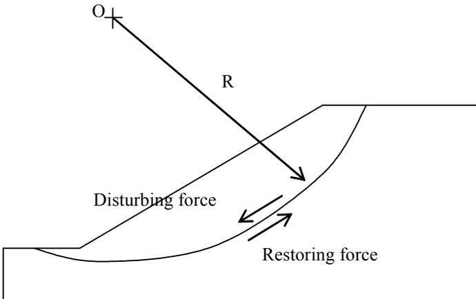
Figure 5-1. Forces acting on a circular slip plane. O is the centre of the slip circle, R is the radius of the slip circle or lever arm.
