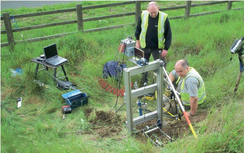
Figure 5-5. Set up of *in situ* shear apparatus (Photo: J.E. Norris).
