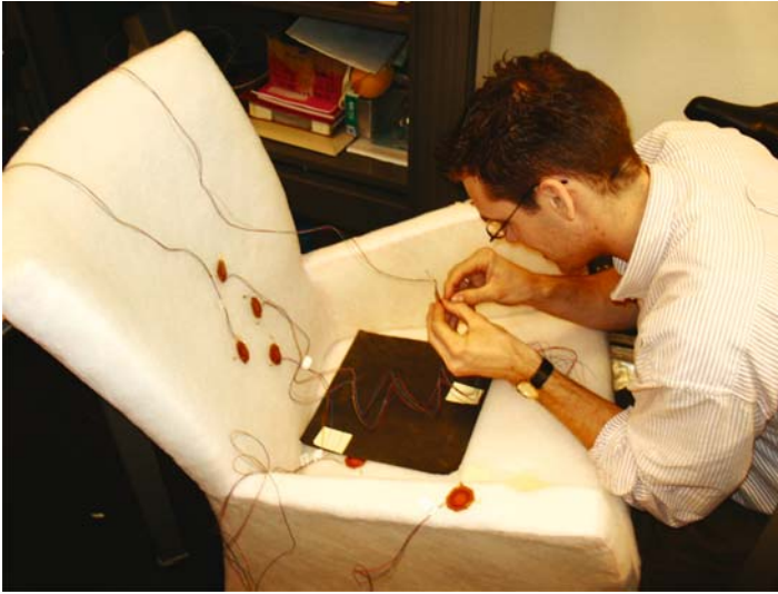
Figure 9. Preparing the sense chair. Amongst the sensor the capacitive groundplane is clearly visible.
