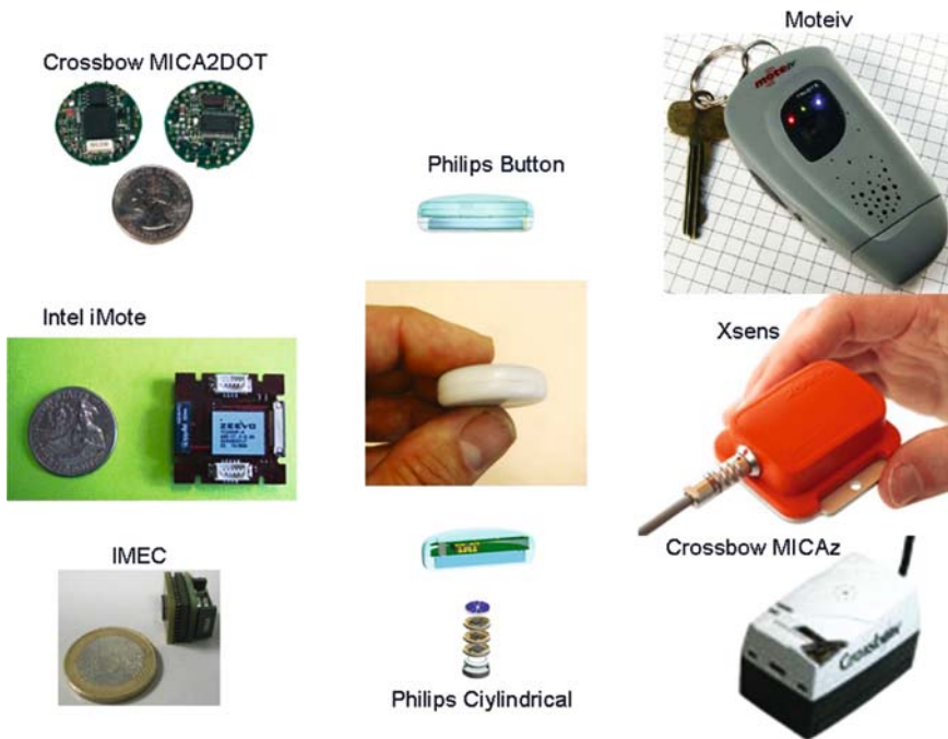
Figure 15. Comparison of the Philips solutions with different devices often cited in the wireless communications community.
