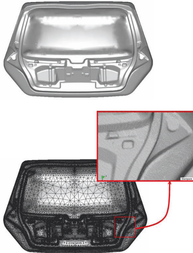
Fig. 13. Car tail gate. Geometry and final adapted mesh of 489560 EBST1 elements used for the stamping simulation
