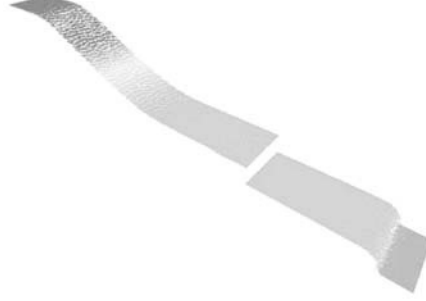
Fig. 10. SDG solution for shock tube example; height and color fields (rendered in gray scale here) indicate density and pressure. Interface tracking delivers sharp resolution of contact discontinuity.
