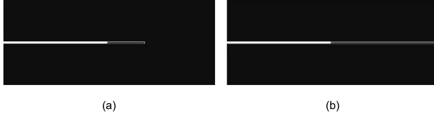
Fig. 5. Final crack path of the element deletion method with a 200 \times 81 quadrilateral mesh at different time steps: (a) t = 30.56 \mu s and (b) t = 65.62 \mu s
