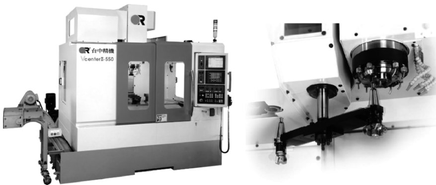
Figure 2.2 A machining center and its automatic tool changer
