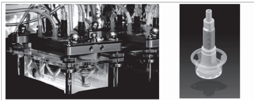
Fig. 31.5 Left: Exposure chamber with three cell culture inserts. Right: 3D image of the aerosol inlet above a Transwell membrane insert with cell culture
