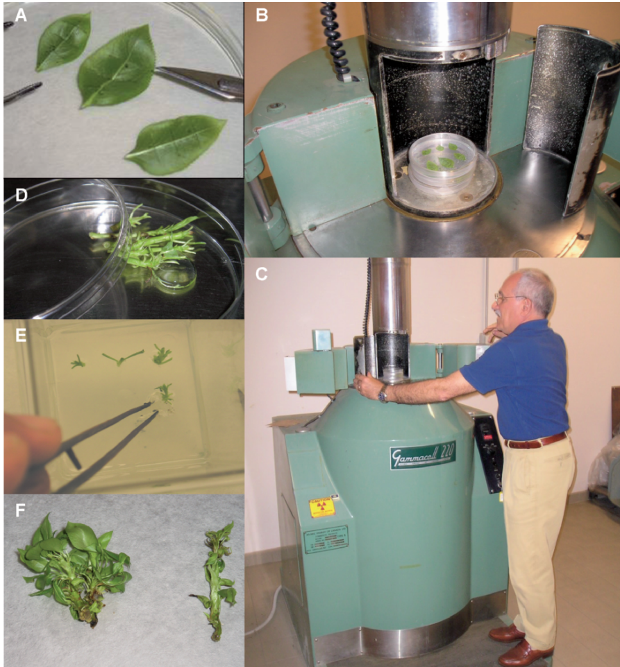
Figure 1. A) Leaves are taken from 30-day-old pear cultures. After three transverse cuts are made to the midrib, leaf blades are placed with the adaxial face touching the regeneration medium. B) Petri dishes containing six leaves each are placed inside a gamma cell for treatment. C) “Gammacell 220” (Atomic Energy Canada Limited, Ottawa, Ontario, Canada) with Petri dishes inside, is closed for having plant material subjected to mutagenic treatment. D) Shoots taken from 30-day-old pear cultures are placed in a Petri dish for treatment. E) After mutagenic treatment shoots are transferred to a fresh proliferation medium. F) Proliferation rate is determined by counting the number of shoots developed from control (left) and from irradiated shoots (right: 60 Gy).
