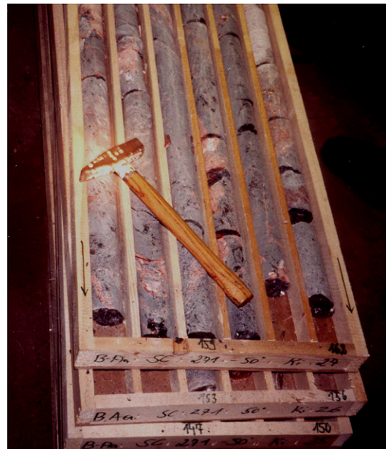
Fig. 2 Drilled bore cores from the salt mine in Altaussee, Austria, obtained from about 500 m below surface. Pink portions represent halite; greyish portions contain mostly anhydrite and some clay
