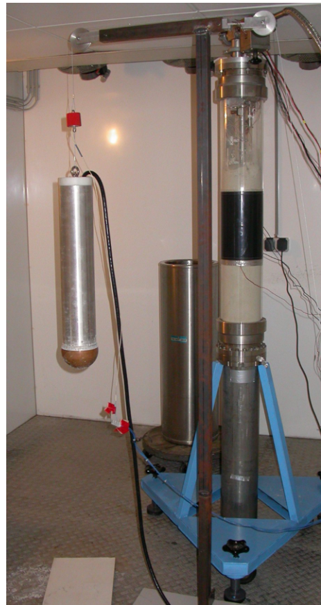
Fig. 3 Setup for melting probe experiments at DLR
