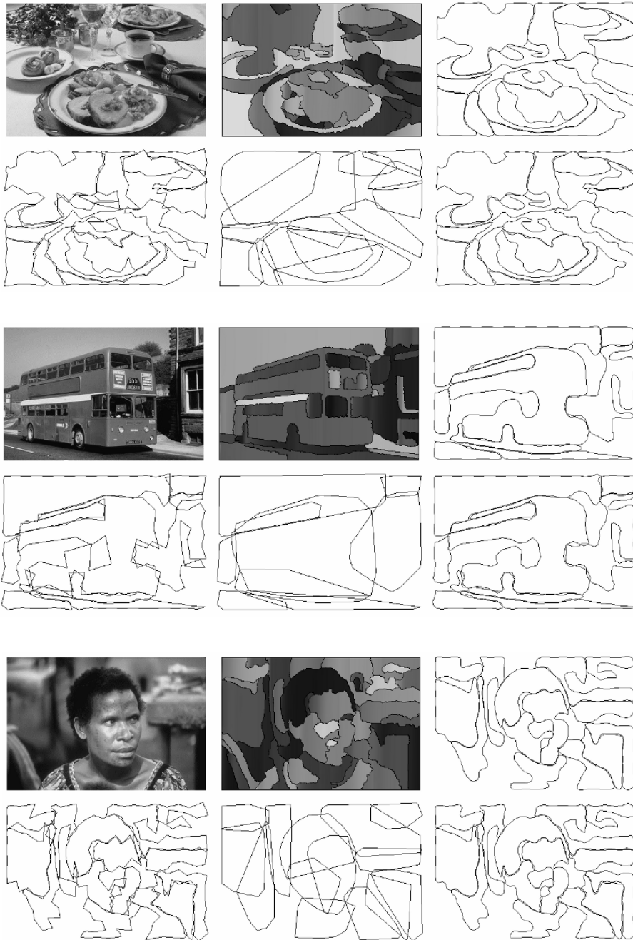
Fig. 6. Top left pictures are original images. Top middle pictures are segmented images. Top right pictures are B-spline approximation. Bottom left pictures show control polygons. Bottom middle pictures show corresponding convex hulls. And bottom right pictures show the one-time refined control polygons after applying Chaikin's algorithm to the control polygons.
