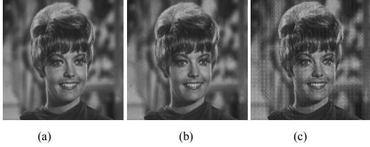
Fig. 2 (a) is the original image “zelda”; (b) is the watermarked image by using the algorithm proposed in this paper; the PSNR is 39.2513. (c) is the watermarked image by using the algorithm proposed in [6], the PSNR is 39.5750.
