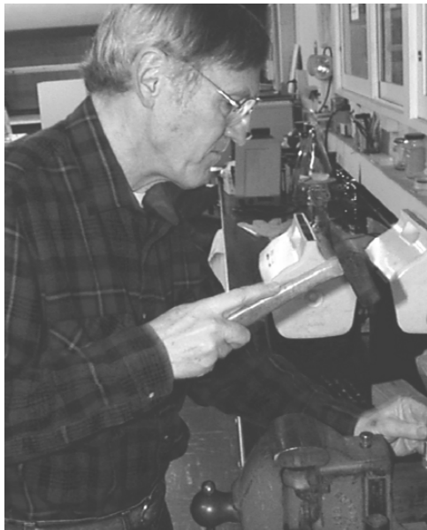
Step 2: Stamp permeation tube body with identification. Weigh the empty body, frit, Teflon window and nut
