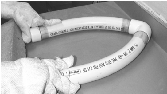
Step 2. After primed pieces are glued and dry, heat to \sim 120^{\circ}\text{C} or until PVC pipe is pliable. Bend pipe by applying steady pressure to top and bottom of canister until legs bow. Set the form by cooling with water
