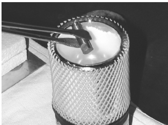
Step 3: Cool permeation tube body in cryogen. Remove cryogen when tube reaches cryogen temperature
