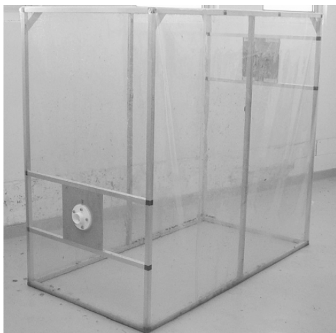
Figure 1. Design of the low-cost open-circuit methane chamber cover. Size (L × W × H): 1.73 × 0.9 × 1.56 m; Frame: 25 × 25 mm square aluminium; Covering: 1.0 mm UV resistant clear flexible PVC sheeting; Chamber air inlet (i.e. front-end): 40 mm PVC flange fitted centrally 50 cm above the floor; Chamber air outlet (i.e. rear-end): 40 mm PVC flange fitted centrally 125 cm above the floor
