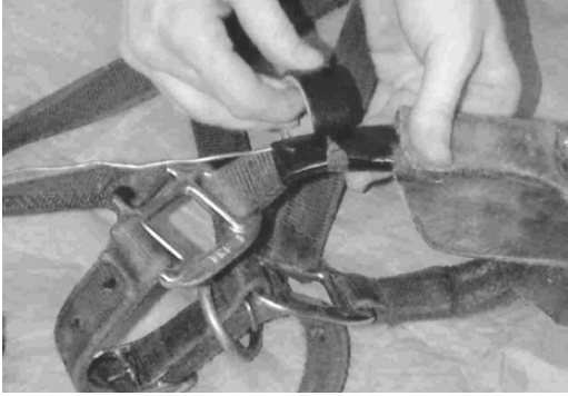
Step 3. Capillary tubing is secured to the halter with electrical (or other) tape
