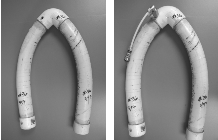
Step 3. Completed PVC collection canister showing the correct location of the tap (left photo) and after addition of sampling valve (right photo). Legs of the collection canister are wrapped in packaging tape to protect against implosion or shattering
