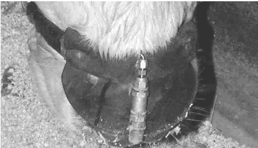
Step 4. After capillary tubing is secured to the halter with tape, the filter assembly is secured to the leather nosepiece with strap ties. Tygon tubing is placed over the end. Note: This photo shows correct location of the filter assembly on the animal's nose
