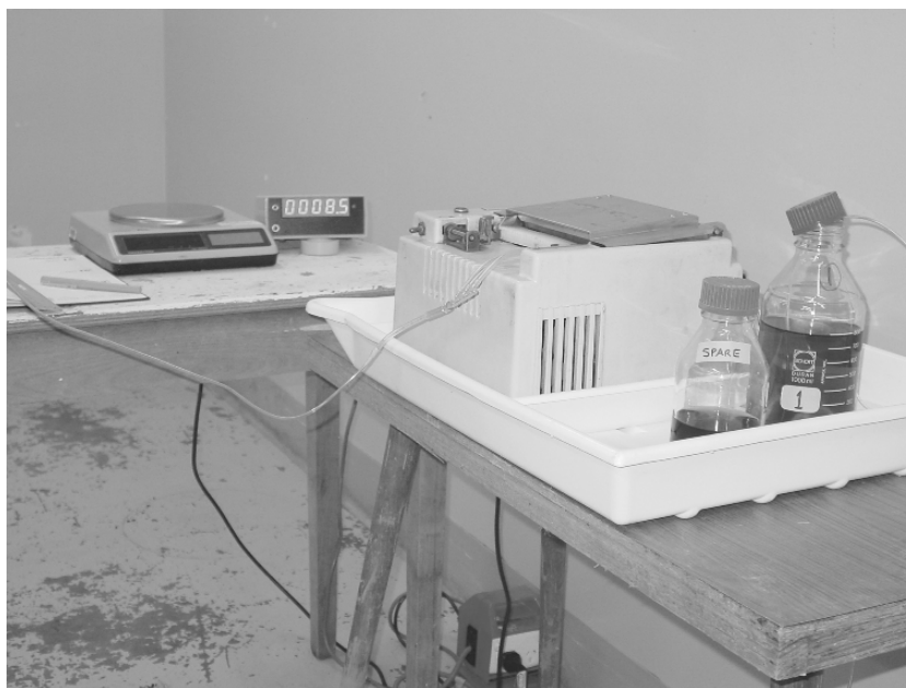
Figure 4. Infusion pump set up for intraruminal infusion. The plastic tray contains the peristaltic pump, an infusion bottled labelled with animal number, a spare bottle of infusate. Scales to determine the weight of infusion bottle, a clock and a data book to record weights, times and comments are nearby
